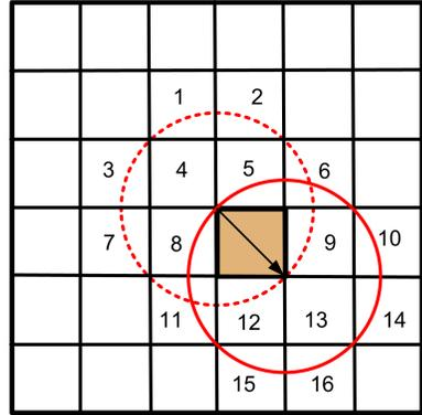
Fig. 2. a) Dividing cell into virtual clusters. b) In the worst case, a good cluster can block at most 16 clusters. In the dashed circle, receiving is not possible and in the solid circle, transmission is not allowed.
