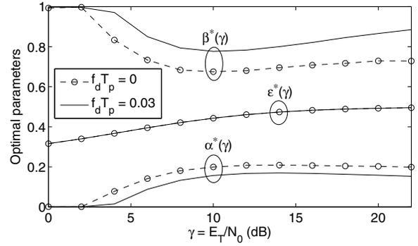
Fig. 6. Optimal values of the parameters of the  $N$ -pilot and  $(N + 1)$ -pilot AS training schemes (8PSK,  $N = 4$ ,  $T_p = 10T_s$ , and  $d = 1$ ).
