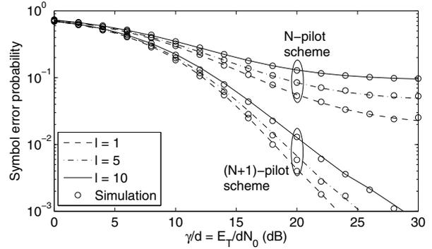
Fig. 3. Comparison of the SEPs of the first, fifth, and tenth data symbols of the  $N$ -pilot and  $(N + 1)$ -pilot AS training schemes (8PSK,  $N = 6$ ,  $T_p = 10 T_s$ ,  $f_d T_p = 0.03$ , and  $d = 10$ ).
