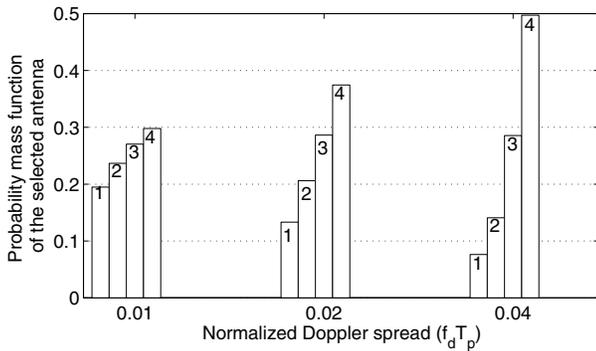
Fig. 5.  $(N + 1)$ -pilot scheme: Probability of selecting different antennas by the optimal affine selection rule for the first data symbol (8PSK,  $N = 4$ ,  $T_p = 10T_s$ , and  $\gamma/d = 20$  dB,  $i = 1$ , and  $d = 50$ ).
