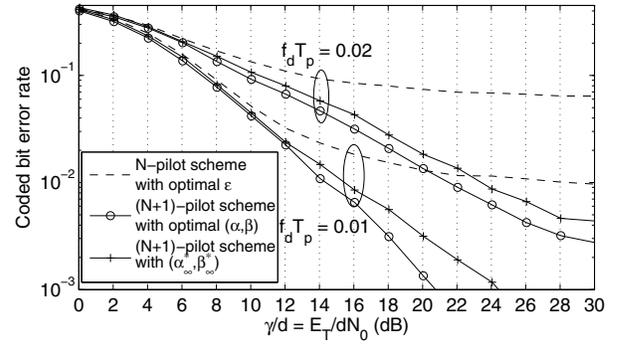
Fig. 9. Performance of  $N$ -pilot and  $(N + 1)$ -pilot AS training schemes for coded packet reception (8PSK,  $N = 4$ ,  $T_p = 10T_s$ , and  $d = 100$ ).
