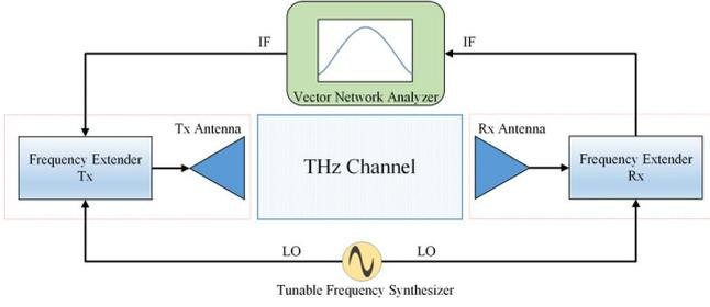
Fig. 1: VNA-based THz measurement setup.
