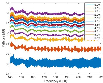
Fig. 4: LoS Measurements for various distances.
