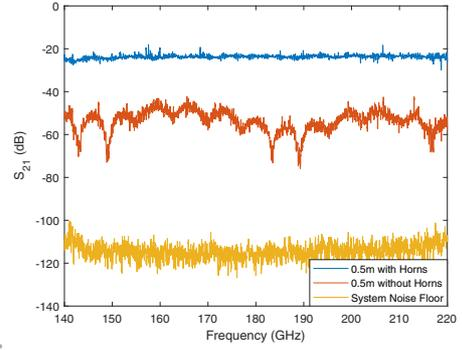
Fig. 2: Comparison of the setup with and without directional horns.
