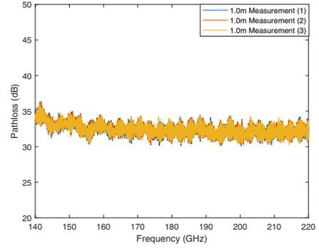
Fig. 5: Measurement-to-measurement variation for one particular distance.
