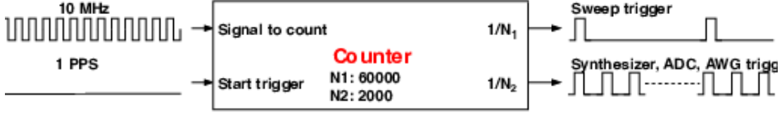
Fig. 4. Operation of the timing module to trigger AWG (TX) or ADC (RX) and frequency synthesizers
