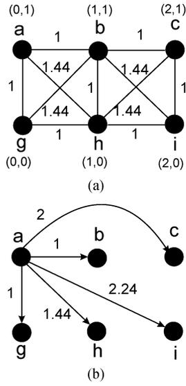
Fig. 1. Construction of graph  $G_h$ . (a) Graph  $G = G_1$  with link costs. (b) Graph  $G(a, 2)$  with link costs.
