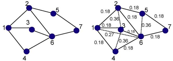
Fig. 7. Left. Wireless network graph,  $G$ . Right. Computation of optimal scheme using super-graph  $G_2$ . The solid edges are those in  $G$ , while the dashed edges are those in  $G_2$  but not in  $G$ . Optimal edge costs are shown for each edge.
