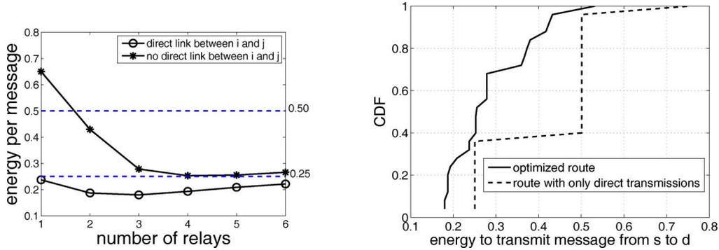
Fig. 8. *Left.* Energy per message for an edge  $(i, j)$  in  $E_2$  when  $(i, j) \in E$  and when  $(i, j) \notin E$ . *Right.* CDFs for energy required to transmit a message from source to destination when optimized local schemes are used and when only direct transmissions are used.
