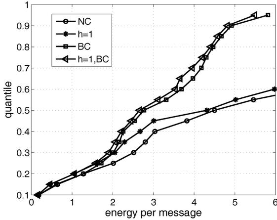
Fig. 3. CDF of energy per message for optimal policies in NC,  $\mathcal{T}_1$ , BC, ( $\mathcal{T}_1 \cup \text{BC}$ ) for a 20-node random network.
