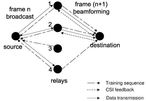
Fig. 6. Broadcast and cooperative beamforming with CSI acquisition process. In frame  $n$ , relays 1, 2, 3, and 4 transmit training sequences to the source, which, in turn, broadcasts the data to relays 1, 2, and 4. These relays then transmit training sequences to the destination in frame  $(n + 1)$ , which feeds back the CSI to relays 1 and 2; these relays beamform to transmit the data to the destination.
