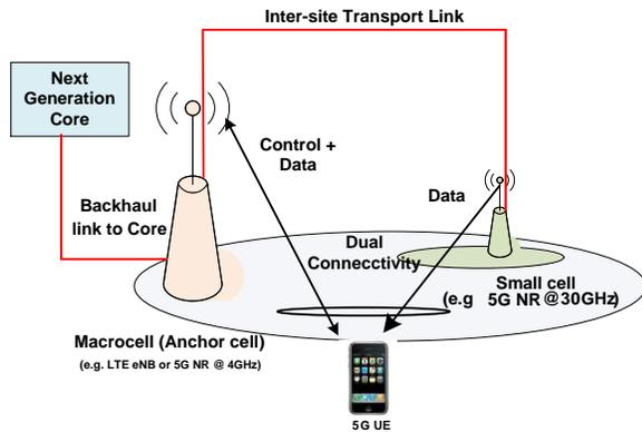
Figure 1. Dual Connectivity Deployment Architecture
