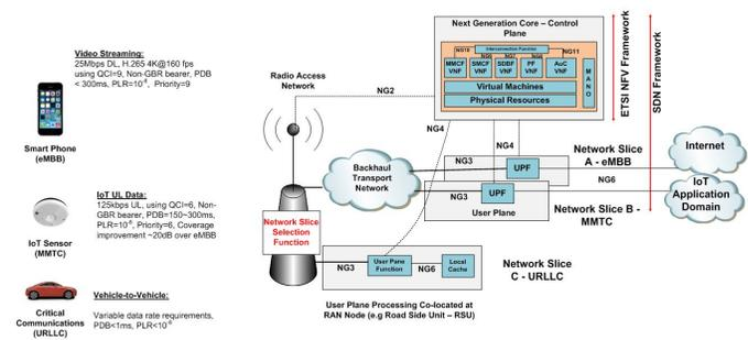
Figure 6. SDN/NFV Supporting 5G Slicing
