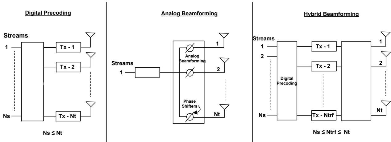
Figure 3. Beamforming Architectures: A. Analog Beamforming, B. Digital Beamforming, C. Hybrid Beamforming.
