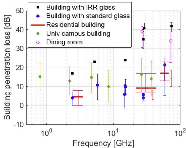
Figure 2. Effective building penetration loss; bars indicate variability for a given building. From [49].
