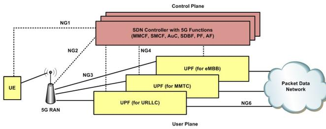
Figure 5. SDN Enabled 5G Core Network
